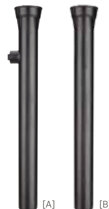
A] PROS-12 B] PROS-12-NSI Overall height: 41 cm Pop-up height: 30 cm Exposed diameter: 5.7 cm Inlet size: ½" Female NPT
