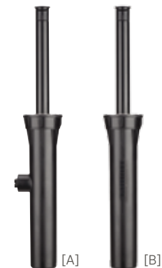
A] PROS-06 B] PROS-06-NSI Overall height: 22.5 cm Pop-up height: 15 cm Exposed diameter: 5.7 cm Inlet size: ½" Female NPT
