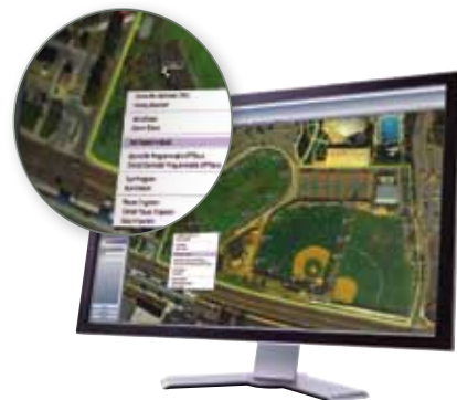
Station level symbols can be positioned over background images from any source.
