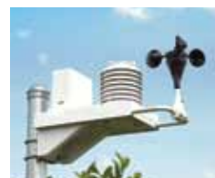
Local ET Sensor, includes Rain Gauge (shown with optional ET Wind anemometer )
